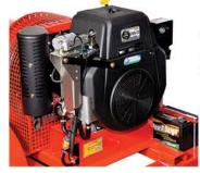
The Agrimetal Turbine Blower is powered by 28 HP SUBARU gas engine.
