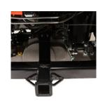
Robust axle mounted hitch with 600 lbs tongue weight and 2,200 lbs. towing capacity (3,500 lbs with trailer brakes)
