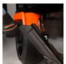
Tool-less access to the radiator and optional hydraulic oil cooler for easy cleaning
