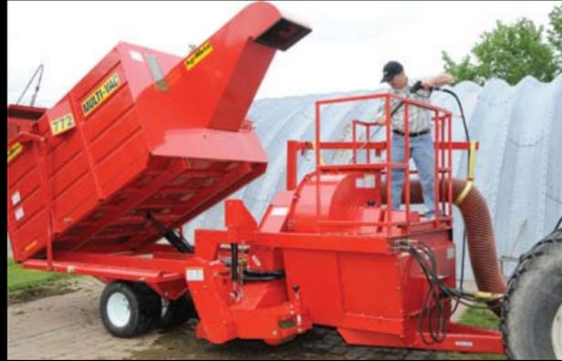
A PLATFORM LOCATED AROUND THE BLOWER HOUSING ENABLE THE OPERATOR TO SAFELY & PROPERLY CLEAN OUT THE INSIDE OF THE BLOWER. A DRAIN TRAP IS LOCATED AT THE BOTTOM OF THE BLOWER TO DRAIN WATER AND RESIDUES. ONCE THE HOPPER IS TILTED, IT IS QUICK AND EASY TO WASH OUT THE INSIDE.
