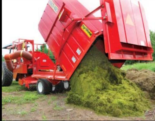
A HYDRAULIC DUMP SYSTEM IS USED TO EMPTY THE DEBRIS FROM THE HOPPER. THE HOPPER TILTS UP TO A 60 DEGREE ANGLE TO COMPLETELY EMPTY THE BOX. THIS SYSTEM IS QUICK AND EFFICIENT ALLOWING THE OPERATOR TO RETURN TO THE FIELD, THUS MAXIMIZING PRODUCTIVITY.
