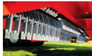
The standard vacuum head of the Multi-Vac may be replaced with a Verti-Tatch head to de-tatch & pick-up debris all in one pass. (spacing 1 1/2 inch cc.)
