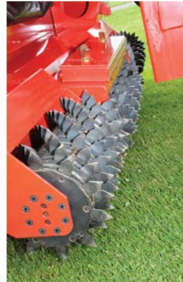
An optional slicer kit can be attached to the Verti-Tatch head. Slicer blades follow the same path as the Verticut blades for deeper penetration. (1 inch x 1 3/4 inch deep) The Verti-Tatch head equipped with a Slicer kit allow you to: de-tatch, collect & aerate fairways all in one pass. This multi purpose pick up head becomes a cost efficient investment because of its year-round use and multiple application. Only 15 minutes is required to switch pick up heads.
