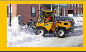
Wille 265 is agile and robust. Its minimum width is 1,200 mm and minimum height 1,990 mm. It weighs only two tonnes, and has operating hydraulics with a flow of 90 lpm. Wille's extensive range of work attachments and tyres makes it a perfect partner.
