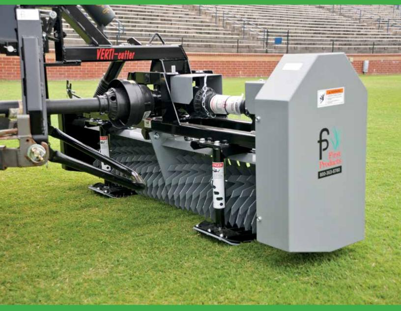
The depth gauge skids are directly centered under the shaft allowing the skids to float over undulations without loosing depth. The skids are preferred in southern type turfs such as Bermudaand zysoia. The replaceable skids systems are made of durable polypropylene.
