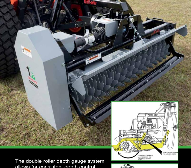
allows for consistent depth control over undulations. The roller offers two big improvements, it prevents marring of the turf and eliminates the forward and rear edge of the skids from digging or pushing up turf which is common in bent grass. With rollers, you can have the option for 1.5" spacing. The rollers are favored in northern turf such as bent grass
