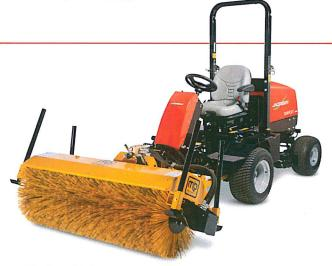
Hydraulic Broom – front-mounted hydraulicallydriven rotary angle broom. Broom speed up to 200 RPM. Storage stands for simple mounting, dismounting and storage.
