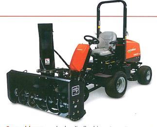
Snow blower – hydraulically-driven two-stage snow blower available in 54", 60" and 72" widths. Up to 40' throw distance and sealed electrical connections with attachment control box.
