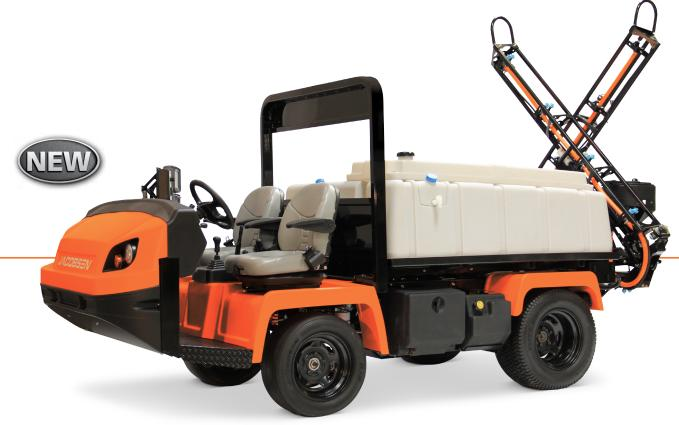
The all-new SprayTek® XP is designed to meet all your spraying needs with precise control. A powerful pump provides ample flow for spraying and agitation and a low-profile tank gives the operator good visibility and the vehicle better handling.
