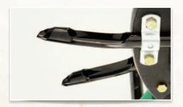
The cast iron aeration wheels have eight tines per wheel standard. Another eight tines can be installed on the wheel doubling the amount of material removed during coring.
