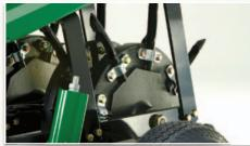
Independently mounted tine wheels follow terrain contours closely for clean, precise aeration of undulated surfaces.
