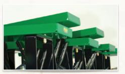
Each weight tray is capable of holding up to 150 pounds for better penetration in heavily compacted soil.
