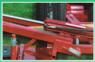
**The main frame wings** are fabricated from heavy wall structural tubing with reinforced high stress areas. All pivot locations are greaseable. All pivot pins are held in place on moving member, thereby eliminating wear.
