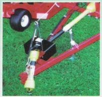
**The input driveline** has two category #6 PTO shafts. This proven system allows for smooth 180 degree turns, easier attachment to tractor, less repairs and maintenance.
