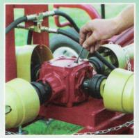
The heavy duty gear box, with machined and case hardened gears, transmits power to the mower decks. All PTO shafts have ring lock collars instead of pins for additional safety. Oil level dip stick and drain plug allow for easy maintenance.
