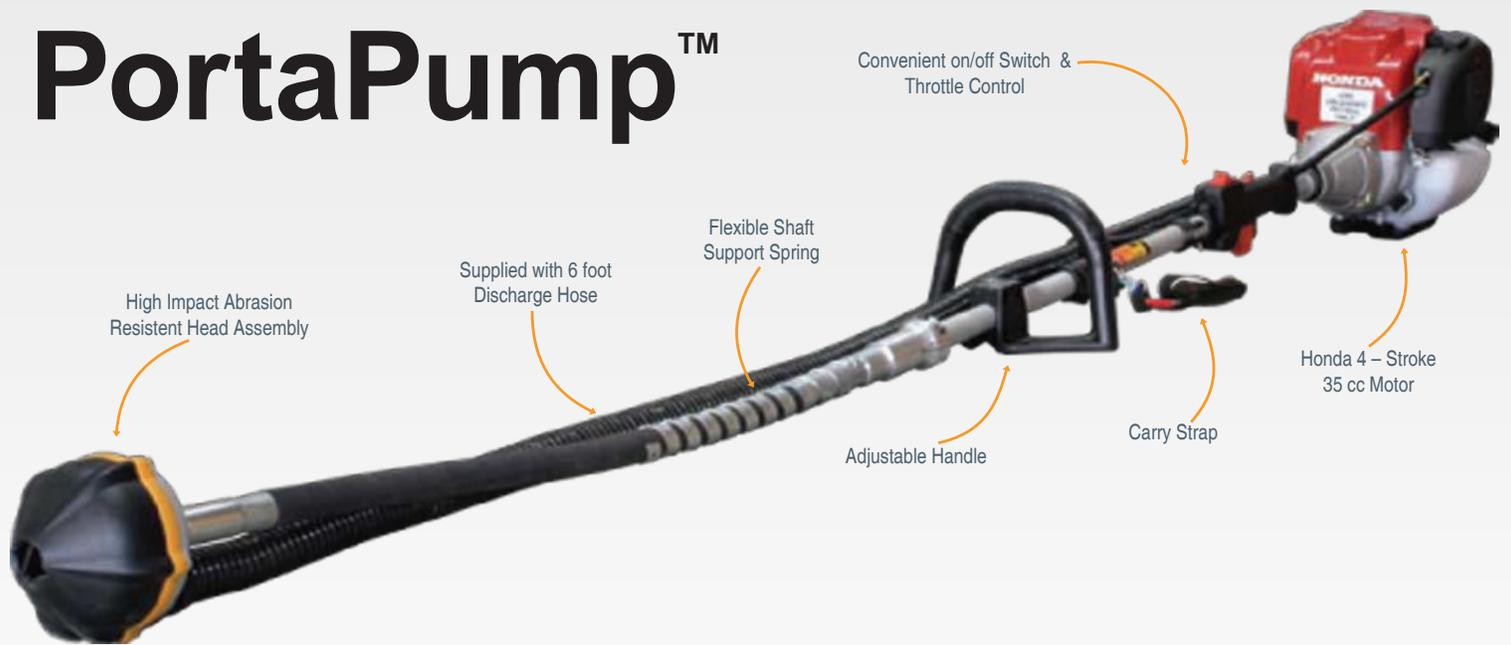
**POWERFUL** – 35cc Honda GX engine powers the 33GPM trash pump. The PortaPump will push water/material through 100' of hose or over a 25' rise without losing pressure. The GX35 Honda engine starts easy, delivers consistent power and runs 90 minutes on a single tank of gas. Cast iron pump impeller insures long lasting performance. The engine, and the PortaPump in total, is backed by a full one-year warranty.
