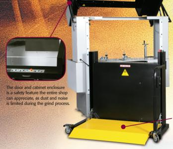
Power...... 115 volts, 60/50 hertz, single phase, 20 amp circuit Grinding Wheel . . . . . Spin: 6" OD x 2.75" ID x 1.5" thick 46 grit type 1
