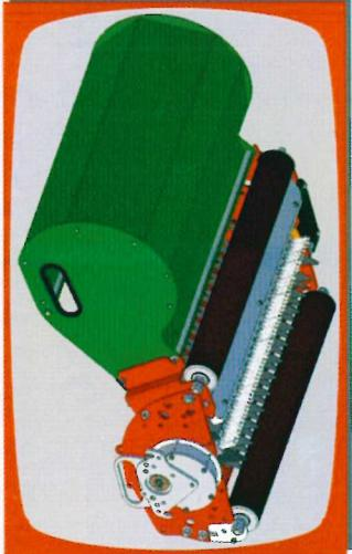
The Counter Rotating Slit Verticutter is a unique attachment for greensmowers, as the main shaft rotates against the drive direction at a reduced speed, due to the special gearbox. The reduced speed increases the torque on the shaft. Because it runs in the counter direction at a lower speed, it pulls out Poa plants and other weeds. Two incorporated brushes clean the surface over the full width.
