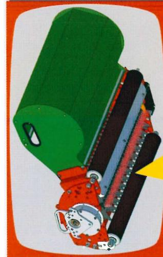
The Counter Rotating Random Verticutter is an innovative attachment. It looks like the GT180, but the (same) blades are mounted at an angle on the main-shaft. Due to this angled blades, every cutting lob cuts its own short slit, close to the nabor one. The depth setting determines the length of the slit and the driving speed determines the number of cuts per square meter. It thinnens the turf, without leaving slits.
