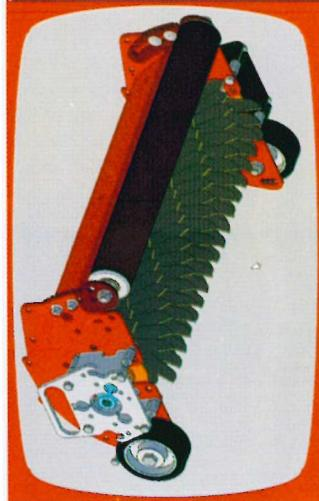
The main shaft of the regular slit verticutter is directly driven by the greensmower motor. It has tipped blades for outstanding lifetime. It does not collect the material, but leaves it on the surface, so it can dry. Next you can blow it off with the sand staying on the green.
