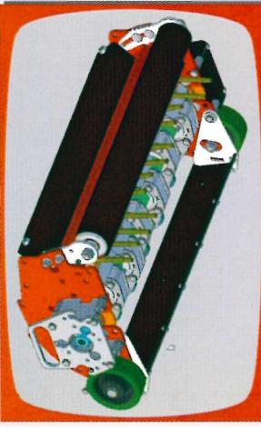
The Recipro Corer has become very popular as thatch remover on greens. It goes 25 mm (1") deep and leaves tiny holes, which are gone in 1-2 days. It is the quickest surface acrifier. The driving speed determines the hole spacing.
