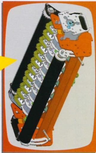
The V-shaped knife sections vibrate due to the driven camshaft. The seed is fed into the vibrating funnels at the rear. The funnels are part of the V-shaped knife sections. So the seed is fed directly into the cut slit and the vibration of the funnels prevent clogging. The accurate seed dosing system is driven by the rear roller. The amount can be set by changing gearheels.
