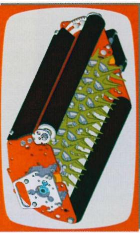
The 6 spike sections roll over the surface and are mounted on a driven camshaft, which add a vibration to the spikes. This vibration creates deep, nice holes. Other tools are available, like disks and thin slicer spikes.
