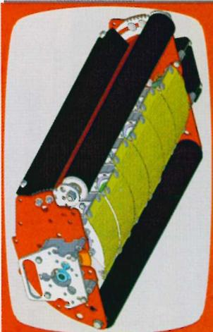
The GT300 works with 6 timed , curved shoe plates, who "walk" over the turf. The depth/ impact can be set by the front roller. Since the 6 sections are well timed, the impact is much more than with a roller. It pushes vertically down. A greenspeed increase of 30% in one pass is possible.
