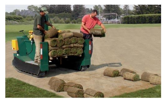
Carries 4000 lbs. with Specialized Heavy Duty Tracks, which minimize disturbance of prepared surfaces. Quickly attach the Standard Forks for pallets or, the Big Roll Attachment, which handles both 42 and 48 inch wide Big Rolls.
