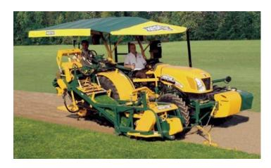
Full Floating Cutter Head, with hydraulic depth control, floats for reliable sod thickness in all ground conditions
