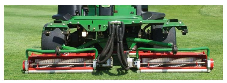
AGRIMETAL GREENS ROTARY BRUSH REPLACES THE REEL MOWER HEADS ON TRI-PLEX GREENS MOWER IN MINUTES. ROTARY BRUSH HEADS FIT IN THE SAME MOUNTS AS THE REEL.
