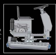
Each floating heads has openings on the top, front and back, making clean up simple. The #80 chain drive system provides ease of operation with years of reliability.
