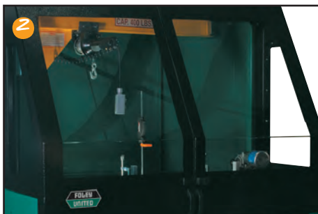
Industrial Cabinetry —helps keep the dust and noise contained in the machine.
