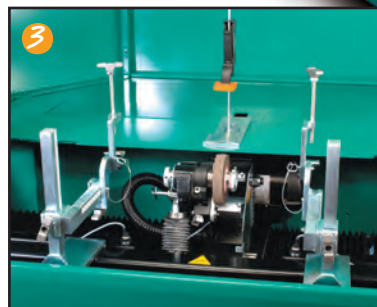
Reel Mounting Brackets —provides quick mounting and dismounting of the reel on a tabletop style base. No tools are necessary for fast and easy repeatable positioning of the cutting unit.
