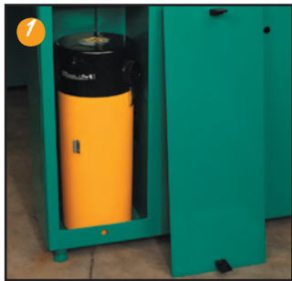
Internal Vacuum System —helps collect the dust and keeps the work area clean inside the cabinet area. All this while keeping the shop dust free!
