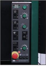
Accessible Control Panel with independent switches for grinding motor, carriage traverse with variable speed control, spin drive with variable speed control, spin/relief selector, variable torque for the "automatic-index" relief process, and a safety stop button.
