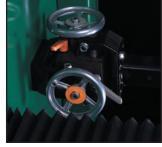
Positive, Vertical and Horizontal Reel Adjustments allows for easy alignment of the reel in the machine so the carriage travels perfectly parallel to reel.
