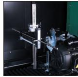
**Dial Indicator Set-Up Gauge** aligns reels within accuracy of .001", establishing the cylindrical quality of the reel before grinding.
