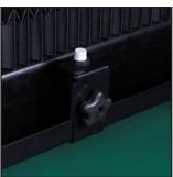
Maintenance Free Electro-Magnetic Traversing Switches are easily adjustable to control the travel length of the grinding carriage.
