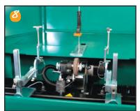
Reel Mounting Brackets—provides quick mounting and dismounting of the reel on a tabletop style base. No tools are necessary for fast and easy repeatable positioning of the cutting unit.
