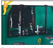
**Electrically Interlocked Guarding**— safety is ensured with doors that keep the operator and others from inadvertently entering the grinding "work" area.
