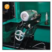
**Spin Drive Unit**—variable speed, reversible, and easy setup accommodates different reel configurations.
