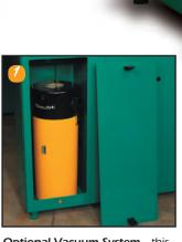
Optional Vacuum System—this option helps collect the dust and minimizes dispersion within the grinding base work area.
