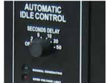
Auto Idle Generator switches to idle mode when no load is present.
