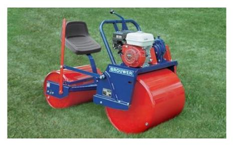
The TR 224 turf roller from Brouwer® is a gentle giant you can trust to start newly laid turf off healthy and strong. This riding roller is easy on turf and easy on the operator, with lever-assist steering, clutchless transmission and single-lever shifting. The TR 224 from Brouwer is a reliable, economical way to set fresh turf.
