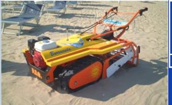
TECHNICAL FEATURES width: 900 mm height: 900 mm length: 1700 mm weight: 310 Kg characteristics
