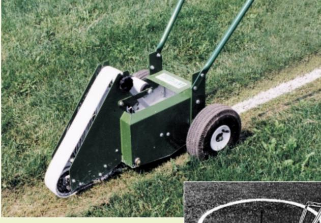
The Bannerman Wet Line Marker is a simple, practical tool for line marking on grass surfaces using low-cost latex paint. A sturdy, well balanced machine with two wide pneumatic tires at the base of the handle, creating a comfortable fulcrum for raising the marking belt
