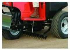
• **Sand Cultivator:** (center mounted) To loosen and precondition crusty and wet sand, and for removing weeds. Covers the full width of the tractor. Operates easily from the seat.
