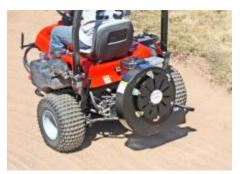
• Engine-Powered Blower: (rear mounted) makes quick work of leaves and debris all over your course. NOTE: Does not fit Diesel Super Star.
