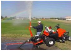
• **Typhoon:** (rear mounted) High-volume pump for liquids and semi-solids. 6.5ft/2m snorkel keeps tractor high and dry. 11 hp/ 8.5kW gas engine with electric start. Removes excess water from bunkers at a rate of 240 gallons per minute. Click <u>here for Spec Page</u>.
