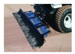
• **Spring Steel Fan Rake:** (rear mounted) For extra-fine smoothing and grooming, and for removing pesky debris like pine needles and leaves.
