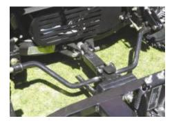
• Qwitch: All rear-mounted implements attach to Smithco Bunker Rakes instantly and effortlessly with the exclusive Smithco "Qwitch" (quick hitch).
