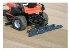
• Tournament Finish Rake: (rear mounted) Applies the finest finish, firmness and playability. Choice of 84" or 72".
