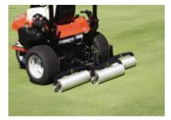
• Roller Brush Spiker System: (rear mounted) 3-section greens. Available in spiker and brush also.
