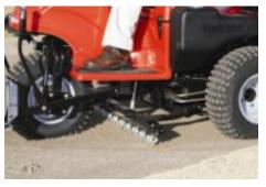
• Spring Tine Sand Cultivator (center mounted) Loosen and pre-condition crusty, packer or wet sand. Easy on turf at bunker edges. Covers full tractor width/ Easily operated from the seat.
