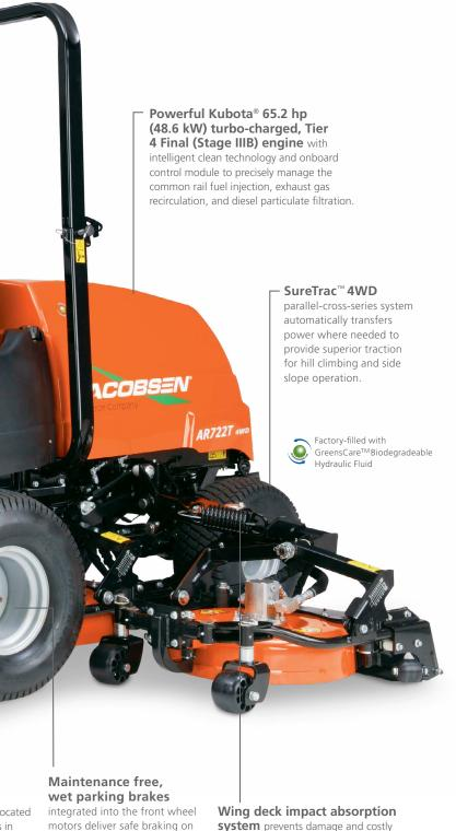
integrated into the front wheel motors deliver safe braking on even the steepest of slopes and have no linkages or pads to service or adjust, reducing total cost of ownership. Wing deck impact absorption system prevents damage and costly repairs. A heavy-duty spring cushions the decks from front impact while the shear pin enables breakaway and quick replacement.
