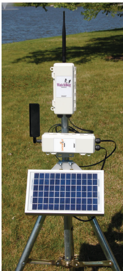
3928M DataScout cellular Modem mounted with a WatchDog Retriever
