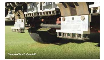
546569 John Deere 800 – Spikes spaced 1¼ in. (3 cm) on center, 48 holes per stroke (Set of 4)
